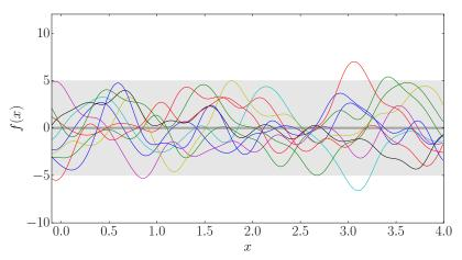
10 samples from the prior distribution using a squared exponential kernel (Eq. 1) with l=0.2 and  $\sigma=2.5$ . The dark grey line indicates m(x), the gray area indicates the 95% confidence region, i.e.  $m(x)\pm 2\sqrt{K(x,x)}=m(x)\pm 2\sigma$ .
