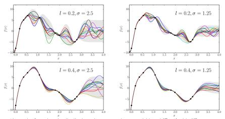
10 samples from the prior distribution using a squared exponential kernel (Eq. 1) with different settings for l and  $\sigma$ . The dark grey line indicates m(x), the gray area indicates the 95% confidence region, i.e.  $m(x)\pm 2\sqrt{K(x,x)}=m(x)\pm 2\sigma$ .
