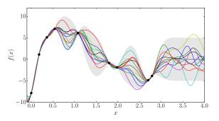
10 samples from the posterior distribution using a squared exponential kernel (Eq. 1) with l=0.2 and  $\sigma=2.5$ . The dark grey line indicates  $\mathbb{E}[f(x)]$ , the grey area indicates the 95% confidence region.
