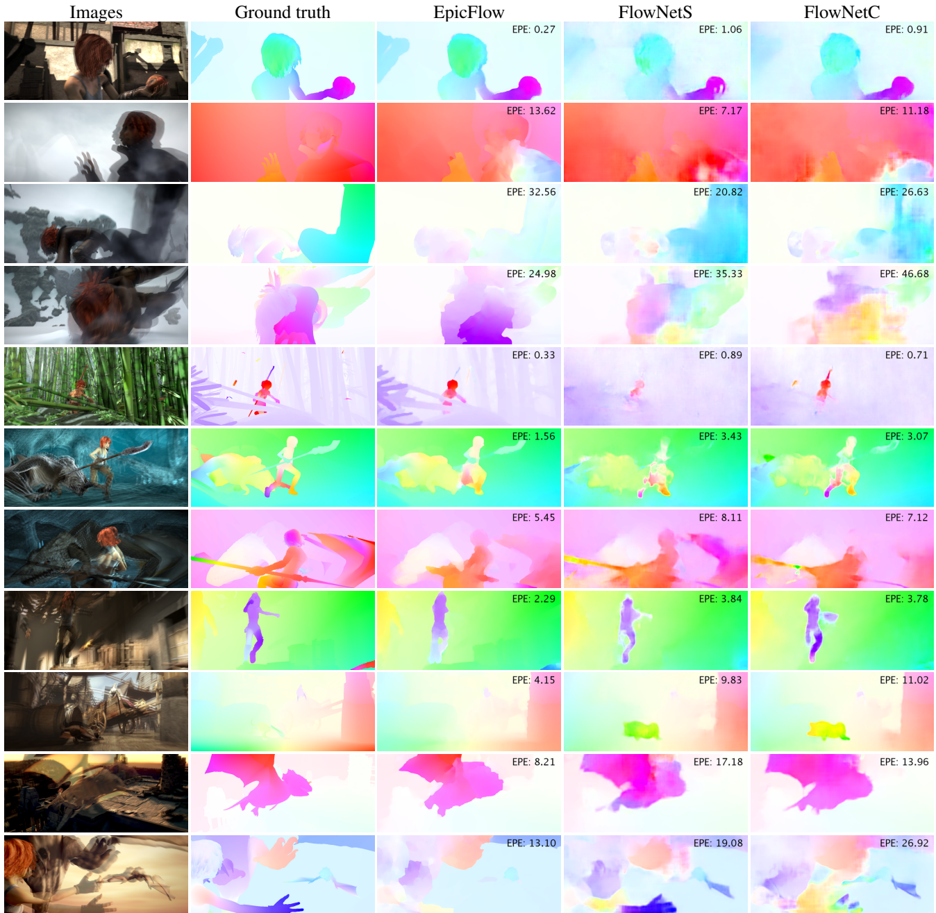
Figure 7. Examples of optical flow prediction on the Sintel dataset. In each row left to right: overlaid image pair, ground truth flow and 3 predictions: EpicFlow, FlowNetS and FlowNetC. Endpoint error is shown for every frame. Note that even though the EPE of FlowNets is usually worse than that of EpicFlow, the networks often better preserve fine details.
