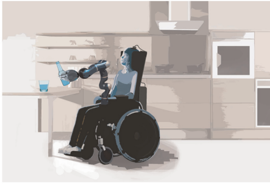
Fig. 1. An assistive torque-controlled robotic hand–arm system to support people with severe physical disabilities.
