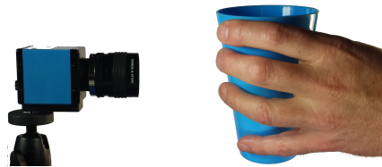
Fig. 1: Setup: a fixed camera observes the fingers to estimate finger grip force and torque.
