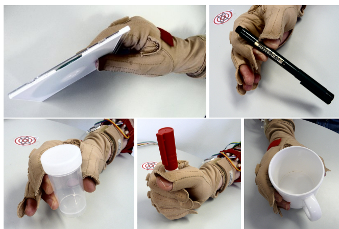
Fig. 2 The five objects while being grasped by a subject: (left to right) flat grasp, pinch grip, tripodal grip, small power grasp and large power grasp. Notice that the subject never pronates and/or supinates the forearm, as instructed.
